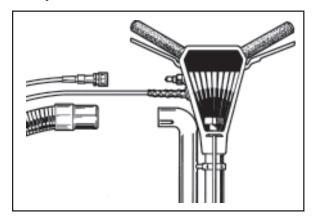
1. Handle Adjustment: Loosen the adjustment knob located below the RX-20 label (turn counter-clockwise to loosen, clockwise to tighten). Adjust the handle to a comfortable height. Several adjustments may be needed before a desirable oper-ating position is found.
