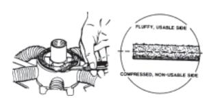
as previously described. Using a pocket knife, carefully pry the seal up and lift it out. If the seal appears worn or glazed so that it will not lubricate well, try turning it over. If that does not work, or if it is damaged, replace it with a new one.
