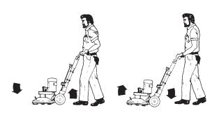
2. Maneuvering Your RX-20: Your RX-20 maneuvers like a rotary floor machine. To move the RX-20 to the right, lift the handle slightly. The more you lift or lower the handle, the faster the RX-20 will move.
