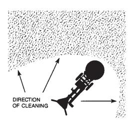
B. The RX-20 is a very aggressive carpet cleaning power head and will leave the carpet with a freshly-cleaned appearance. The carpet should be brushed or groomed after the cleaning process to remove any swirl marks left behind.
