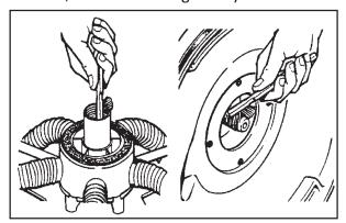
8. Lubricate the felt vacuum seal on top of the hub with a quality,
