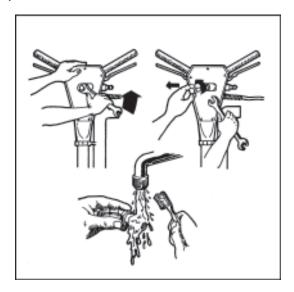
5. Check the jet spray for evenness. An uneven spray will cause improper flow of the cleaning solution.
